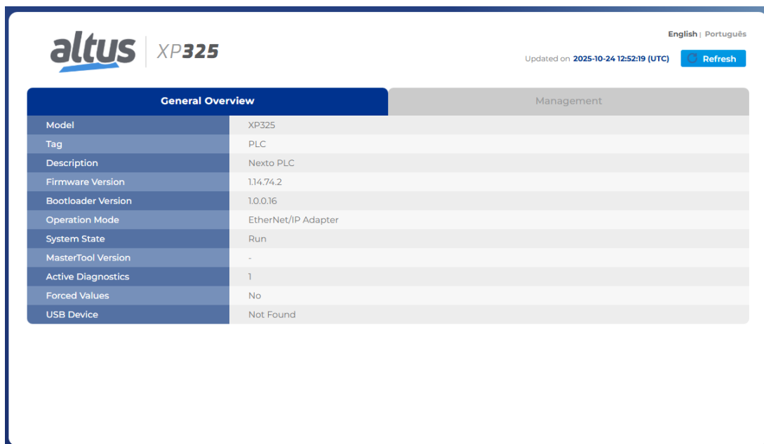
Figure 153: Operation Mode in the PLC Overview Screen
